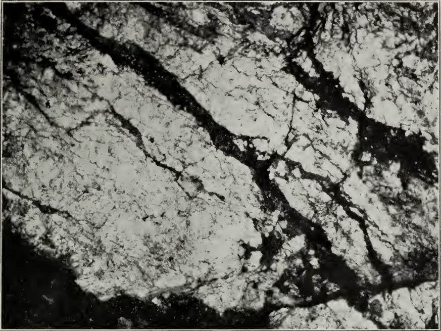
FIG. 21. Calcite vein material traversed by irregular veinlets of fluorite (black). Hillside Mine, 350-foot level, about 250 feet south of the shaft cross-cut. The field shown is about 4 feet across.
